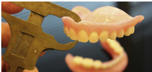
Fig. 14. A denture is measured from the incisal/occlusal surface to the intaglio surface opposite that tooth. This is the entire distance energy will be absorbed by the materials before reaching the attachment. If the amount of material within the distance measured is less than ideal, the denture will break. Table 8 shares minimum distances from incisal/occlusal surfaces to the residual ridge to help provide sufficient material bulk to avoid prosthetic breakage.
